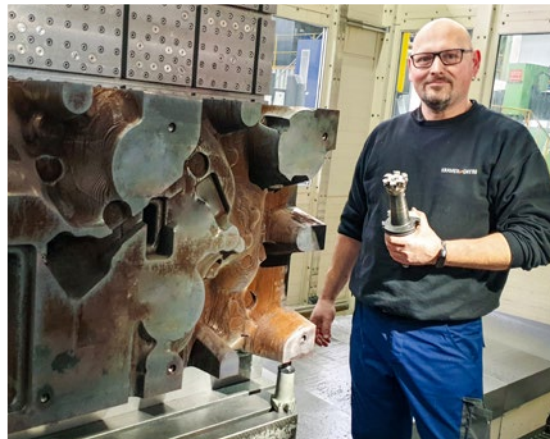
Machine operator Michael Lauber with the NeoMill-4-HiFeed-90 at a mould clamped and ready for machining.
