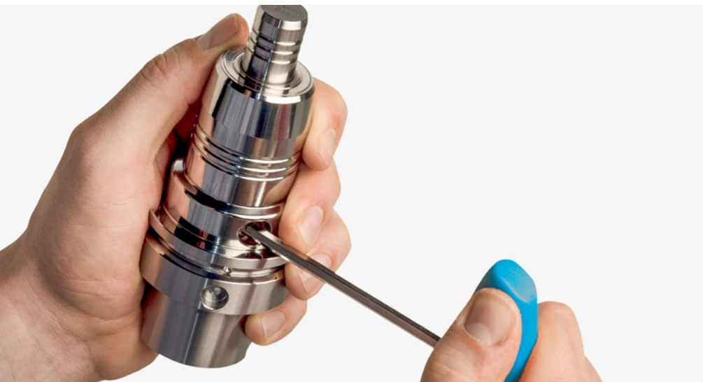
All hydraulic chucks are very easy to use. Tool changes are done in seconds and with micrometre accuracy without peripheral devices. ©SCHUNK
