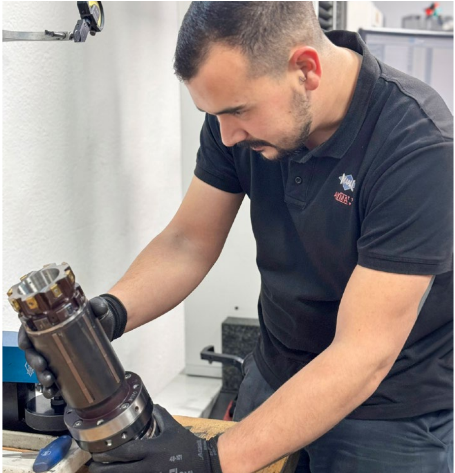
Agustin Calado (MAPAL Tool Setter) inspects the HPR400 with new indexable inserts for fine machining crankshaft bearing journals on engine blocks.
