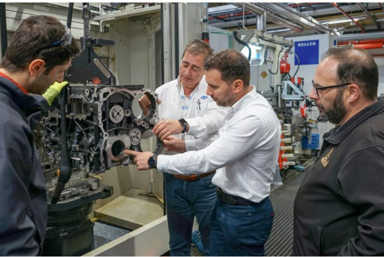
Inspection of the machining quality on a prototype of the engine block for DEUTZ's 3.9-litre engine (left to right): Jorge Montaño (Process Technician), Juan Jesus Roldan (MAPAL Engine Block Technician), David Castaño (MAPAL Tool Manager) and Armando Gutierrez (Quality Engineer).
