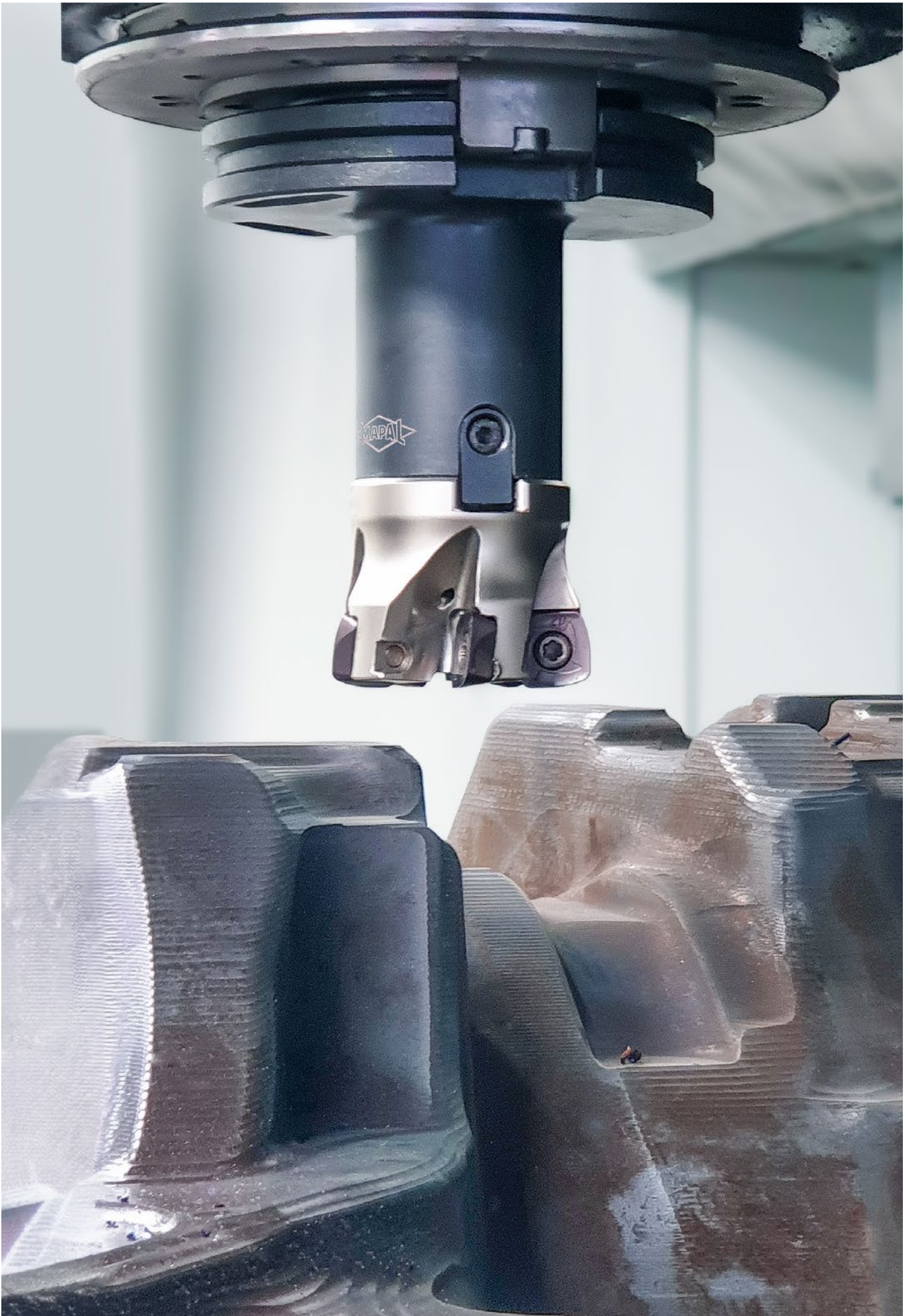
Krämer+Grebe uses a six-bladed NeoMill-4-HiFeed-90 for roughing moulds.
