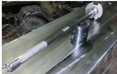
Cooperation between Krämer+Grebe and MAPAL began with a 600-mm-long reamer needed to manufacture low-pressure moulds.
