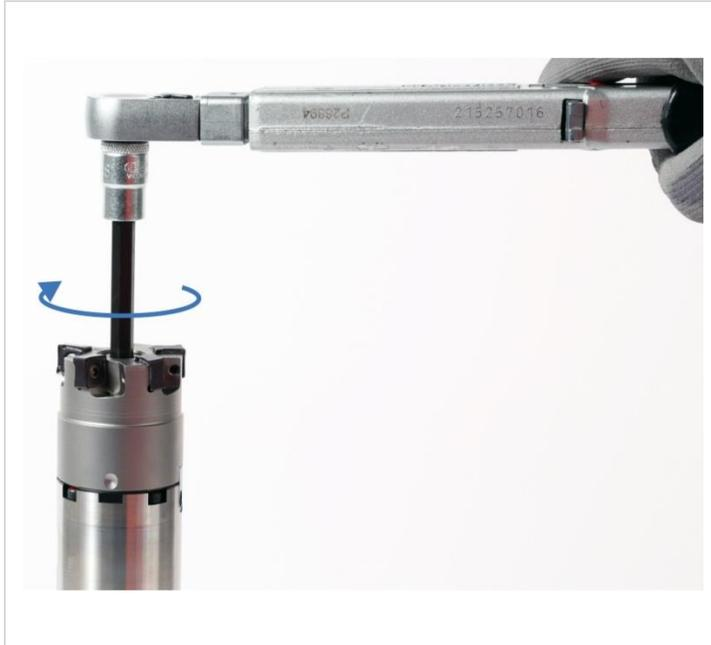
Fig. 5: Tighten the milling cutter clamping screw
