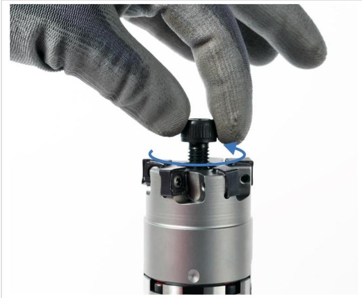
Fig. 7: Removing the milling cutter clamping screw
