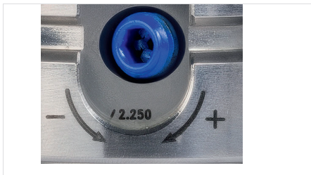
Fig. 6: Marking for checking of the clamping force: Three possible positions on the clamping chuck
