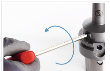
Fig. 12: Loosening clamping screw
