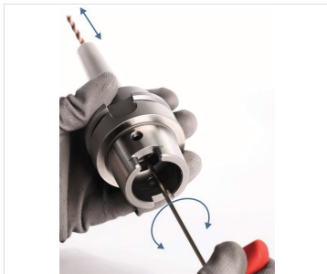
Fig. 10: Adjusting the tool length
