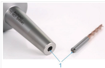
Fig. 8: Cleaning hydraulic chuck and tool
