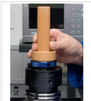
Fig. 10: Cleaning the HSK interface
