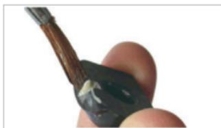
Fig. 16: Greasing clamping jaws
