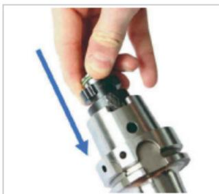
Fig. 20: Testing KS clamping cartridge
