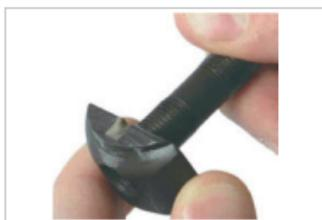
Fig. 17: Screwing the threaded spindle
