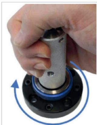
Fig. 9: Arresting the KS clamping cartridge
