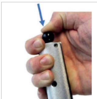
1. Open the KS assembly pliers gripper jaws by pushing down the ball head.
