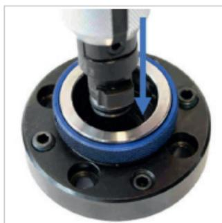
Fig. 8: Inserting the KS clamping cartridge
