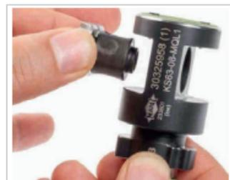
Fig. 24: Fitting the clamping jaw (3)
