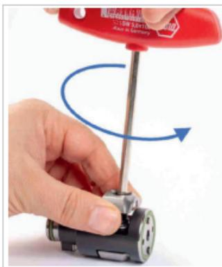
Fig. 26: Screw in the threaded spindle
