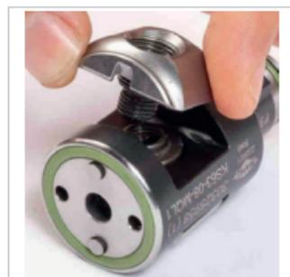
Fig. 25: Fitting the threaded spindle
