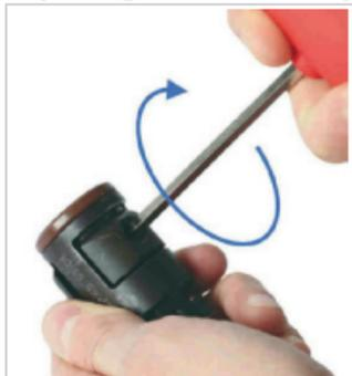
Fig. 15: Disassembling the KS clamping cartridge
