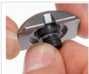
Fig. 23: Screwing the threaded spindle
