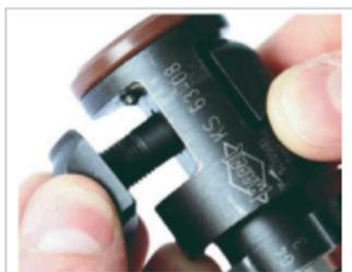
Fig. 18: Fitting the threaded spindle
