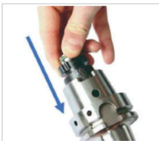
Fig. 27: Testing KS clamping cartridge
