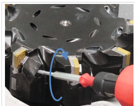
Fig. 10: Tightening the clamping jaw
