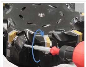
Fig. 14: Tightening the clamping jaw
