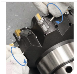
Fig. 6: Loosening the clamping jaw
