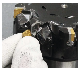
Fig. 8: Removing the indexable insert
