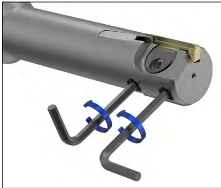
1. Turn both threaded pins 1/2 turn anticlockwise.
