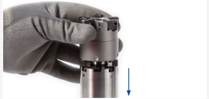
2. Clamp the milling cutter arbor in a changing device.
