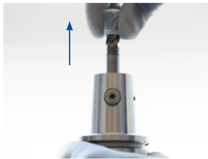
2. Remove the tool from the mill chuck's location bore.
