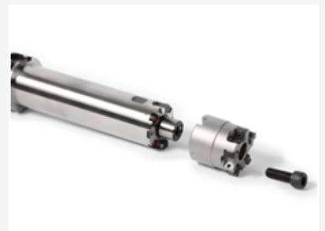
3. Remove the tool from the milling cutter arbor.
