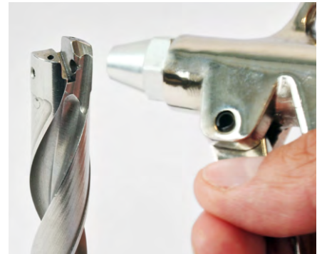
3. Clean the insert seat using compressed air.
