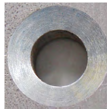
Countersink with extremely unequal spacing
