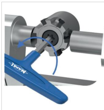
Abb. 24: Justierelement lockern
