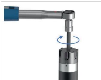
Fig. 12: Tightening threaded spindle to tightening torque
