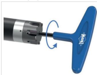
Fig. 17: Undoing threaded spindle
