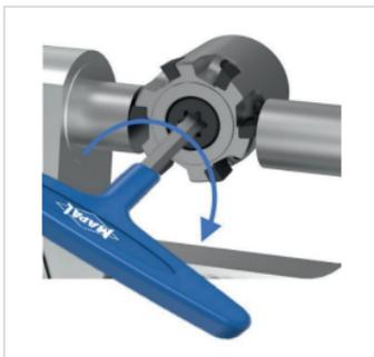
Fig. 23: Adjusting final dimension
