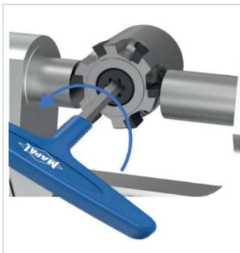
Fig. 24: Loosening the adjustment element
