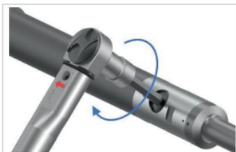
Fig. 16: Tightening clamping stud to tightening torque
