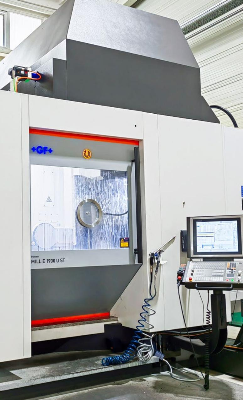
The 5-axis milling centre MILL E 1900 U ST used for machining prototypes made of high-strength cast iron with spheroidal graphite.
