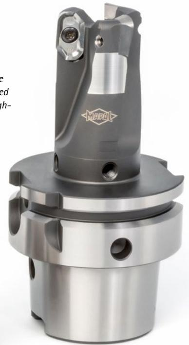
**2** *The OptiMill-Alu-Wave is a new and improved version of the solid carbide roughing cutter from MAPAL. For the tests, the milling cutter with the largest available diameter of 25 mm was used and ran with a spindle power of up to 175 kW. It achieved a material removal rate of 20 dm<sup>3</sup>/min. © bavius*
