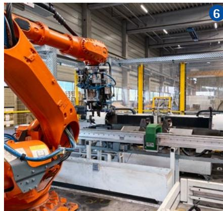
**3** Mössner developed the system for machining round steel bars specifically for the requirements of GABO STAHL.
