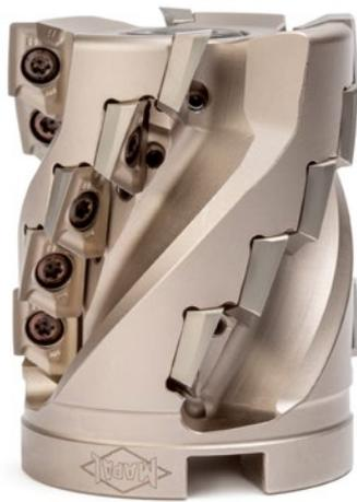
*The shell end face milling cutter NeoMill-Titan-2-Shell performs trochoidal milling convincingly with maximum machining rates, very quiet running and optimal chip removal.*
