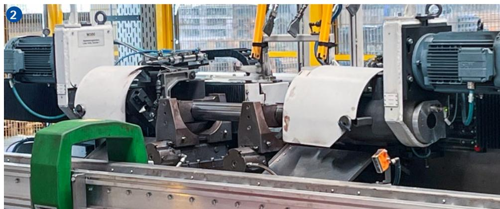
2 The round steel bars are machined on both sides at the same time.
