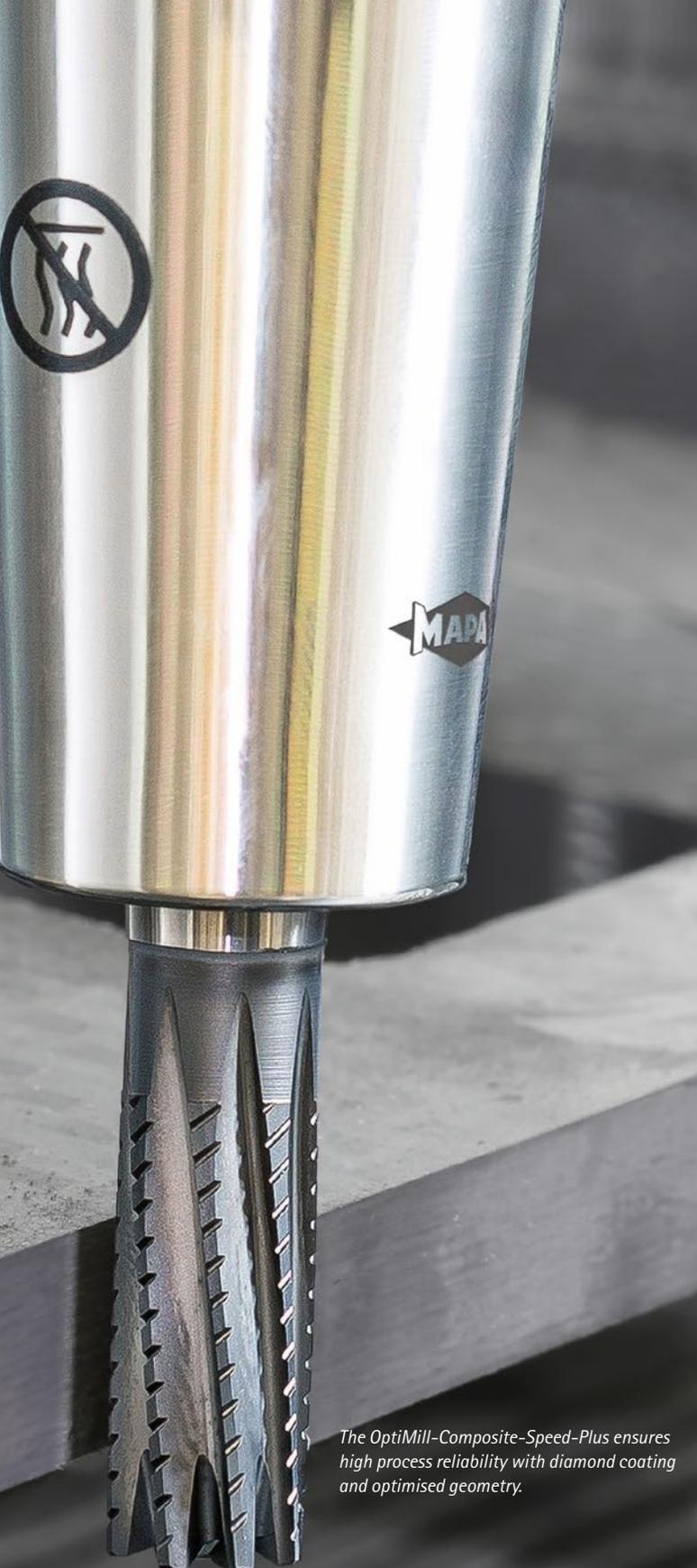
*The OptiMill-Composite-Speed-Plus ensures high process reliability with diamond coating and optimised geometry.*
