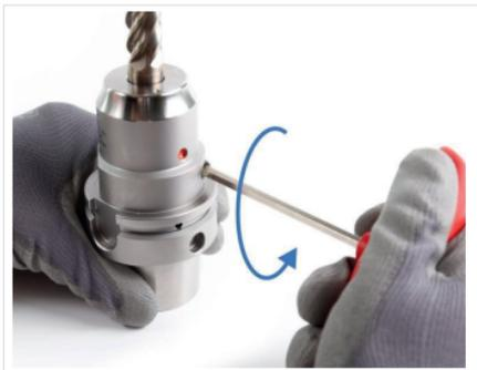
Fig. 12: Loosening clamping screw
