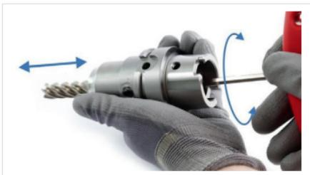
Fig. 8: Adjusting tool length (axial)
