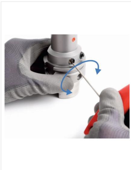
Fig. 10: Adjusting tool length (radial)
