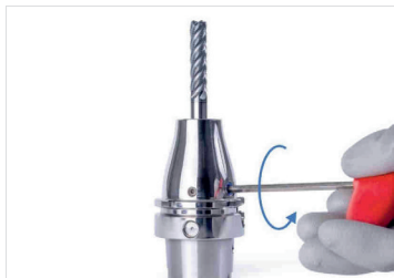
Fig. 12: Loosening clamping screw
