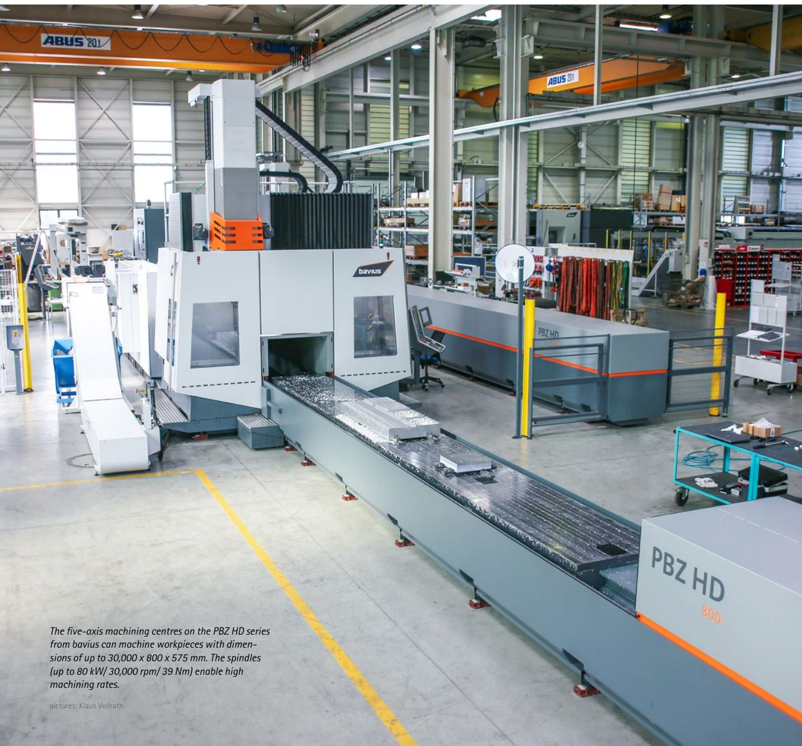
*The five-axis machining centres on the PBZ HD series from bavus can machine workpieces with dimensions of up to 30,000 x 800 x 575 mm. The spindles (up to 80 kW/ 30,000 rpm/ 39 Nm) enable high machining rates.*
