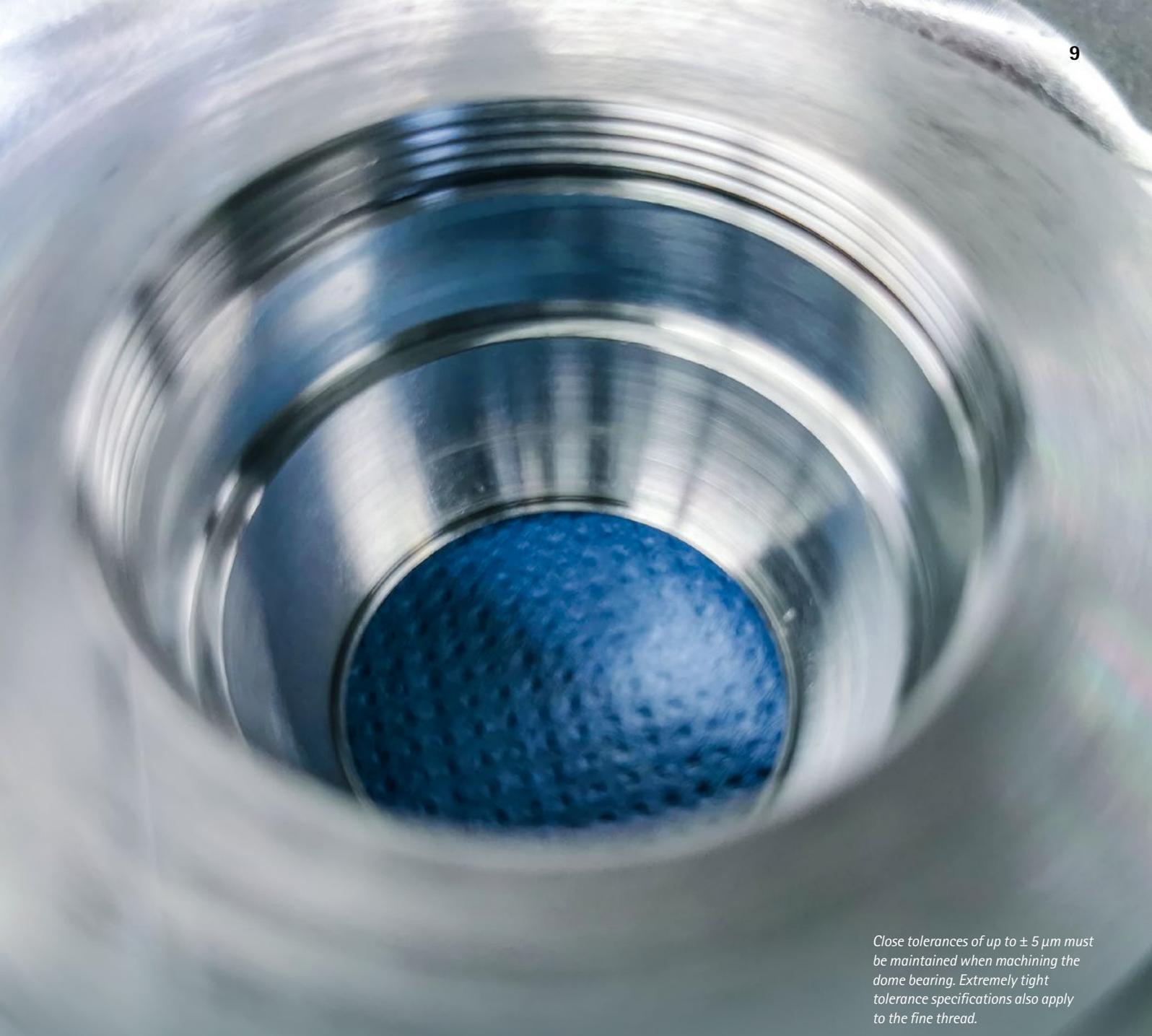
*Close tolerances of up to  $\pm 5 \mu\text{m}$  must be maintained when machining the dome bearing. Extremely tight tolerance specifications also apply to the fine thread.*
