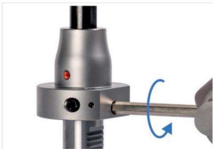
Fig. 18: Loosening locking screw
