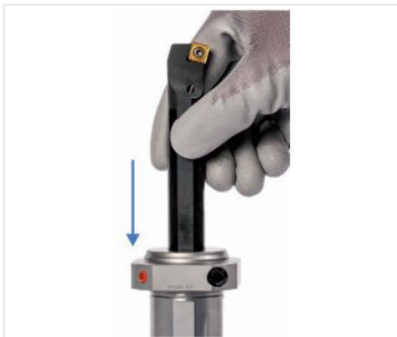
Fig. 19: Inserting tool
