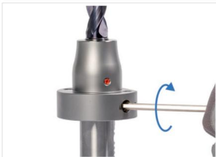
Fig. 11: Tightening clamping screw 2
