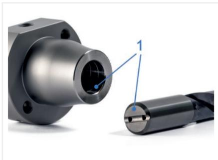
Fig. 7: Cleaning hydraulic chuck and tool
