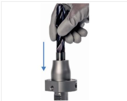
Fig. 10: Inserting tool
