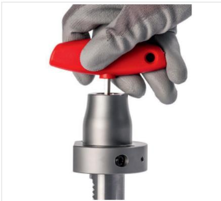
Fig. 8: Adjusting tool length (axial)
