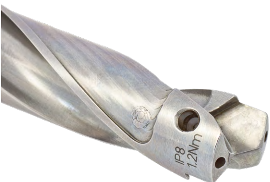
4. Fit the new indexable insert in the insert seat. Hand tighten the special clamping screw using the supplied TORX® PLUS wrench by turning it clockwise.
