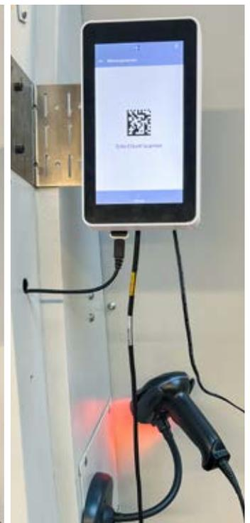
Two of the EMCO machines are equipped with c-Connect boxes for transferring data via scan to the machine.
