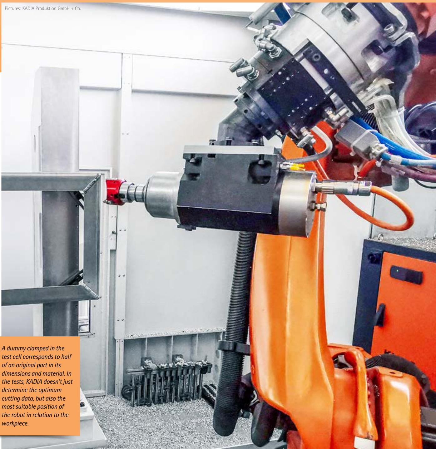
*A dummy clamped in the test cell corresponds to half of an original part in its dimensions and material. In the tests, KADIA doesn't just determine the optimum cutting data, but also the most suitable position of the robot in relation to the workpiece.*
