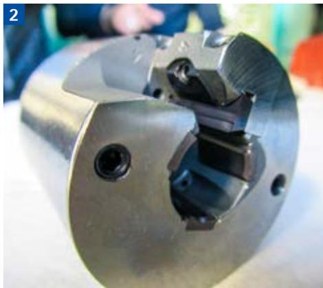
2 The conventional tool for external reaming with three guide pads and the indexable insert with one cutting edge.
