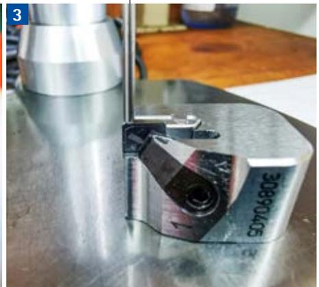
3 The cassette's flat bottom is the reference surface for quick and easy setting of the insert position.
