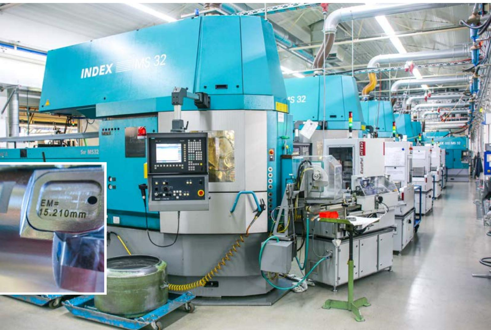
*Multi-spindle automated lathes stand side by side in the machine hall.*
