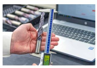
At just the touch of a button, measurement results are transferred from the Bluetooth caliper to c-Com.
