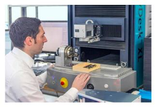
The DataMatrix codes required for the unique identification of the tools are applied to the tools at MILLER using a laser system.
