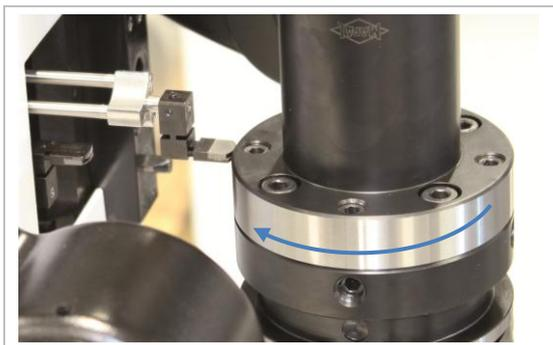
Figure 9: Radial run-out check on the KS flange adapter
