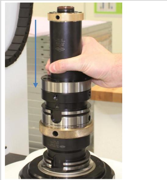
Figure 4: Inserting the KS flange adapter
