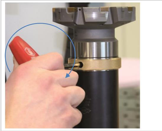
Figure 7: Tightening the clamping screw of the HSK connection
