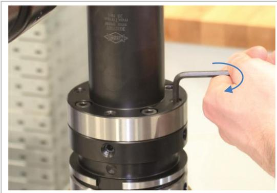
Figure 16: Tightening the axial angular alignment screws exactly
