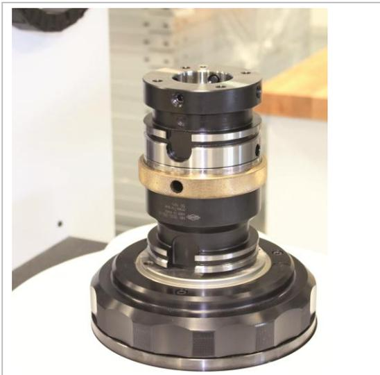
Figure 3: HSK adapter in the connection of the setting fixture
