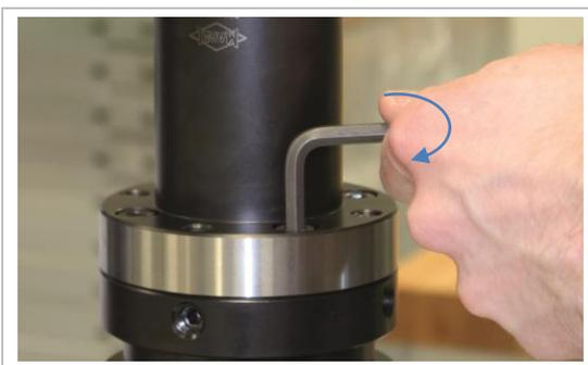
Figure 17: Tightening the axial fastening screws exactly
