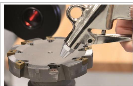
Figure 20: Cleaning the insert seat with compressed air
