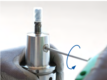
1. Loosen the clamping screw by turning it anticlockwise.
