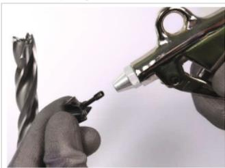
Fig. 5: Clean with compressed air
