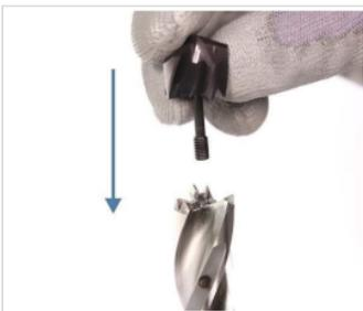
Fig. 6: Fit the replaceable drill head
