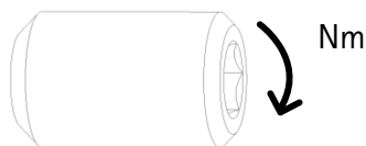
Figure 28, Threaded pin for clamping cartridges, ISO tools, fine boring tools and adaptors
