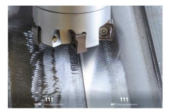
The new milling cutter arbors with vibration dampening enable significantly better surface finishes during machining. The image shows in direct comparison on the left milling paths without vibration dampening and on the right with vibration dampening.
