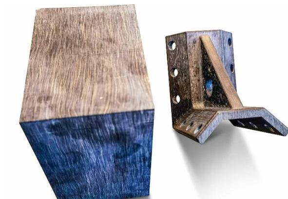
Solid, 100 mm thick CFRP block made of EPRATEX\_CFS 100 and the test component produced from it by milling. ©MAPAL
