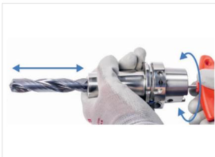
Fig. 12: Adjusting tool length (axial)
