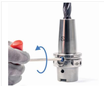
Fig. 14: Loosening clamping screw
