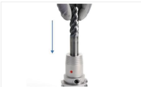
Fig. 8: Inserting tool
