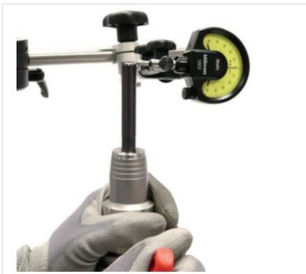
Fig. 17: Adjusting the radial run-out
