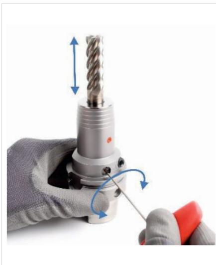
Fig. 11: Adjusting tool length (radial)
