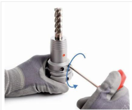
Fig. 13: Loosening clamping screw
