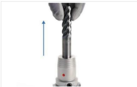
Fig. 14: Removing tool
