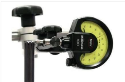
Fig. 16: Measuring the radial run-out
