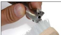
1. Clean the TTS connection on the tool holder with a brush.
