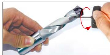
2. Undo the clamping screw with the aid of the hex wrench supplied.
