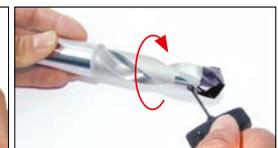
3. Tighten hand-tight the clamping screw by turning clockwise.
