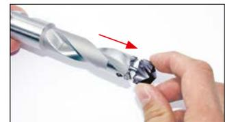
3. Pull the drill head out of the serration.
