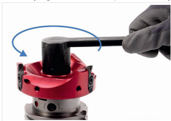
Fig. 8: Loosening the milling cutter clamping screw
