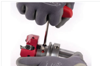
Fig. 9: Loosening clamping screw
