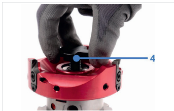
Fig. 5: Screwing in the milling cutter clamping screw
