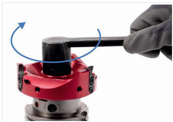
Fig. 7: Tighten the milling cutter clamping screw
