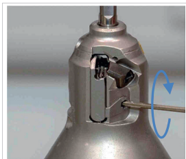
Fig. 16: Tightening clamping screw
