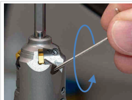
Fig. 4: Loosening the clamping screw
